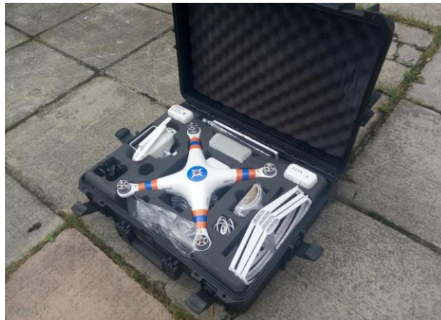
Pict. 1. Phantom 3 Professional unmanned aerial vehicle
